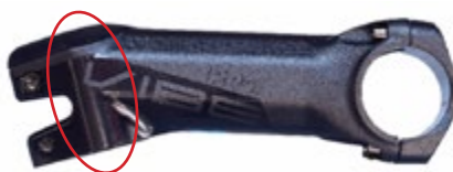
Figure 2: Cracking can occur in the clamping area of the fork steerer tube.
